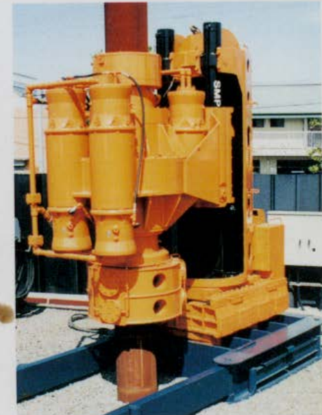
Steel Pipe Piler
