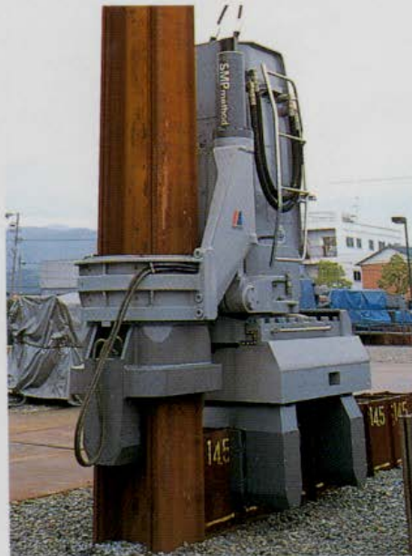
Silent Piler for H-section Steel Piles Only
